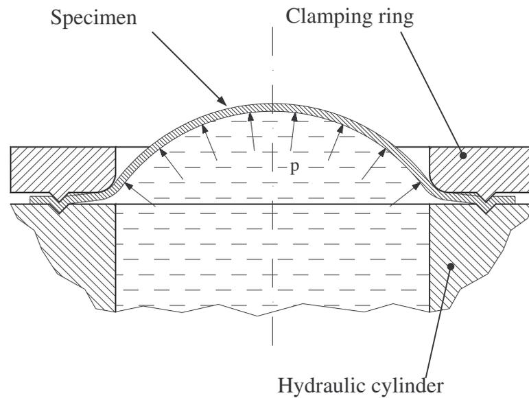
Figure 1. Hydraulic bulging test
