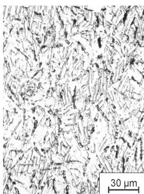
Fig. 5. Microstructure of TiAl6V4 after hot forming
