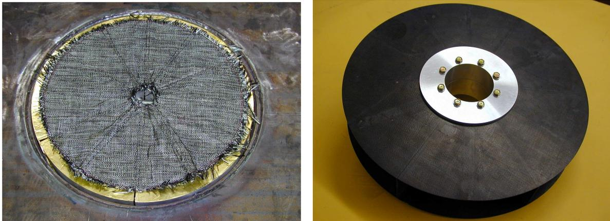
Fig. 7. Textile rotor preform with tool and consolidated rotor
