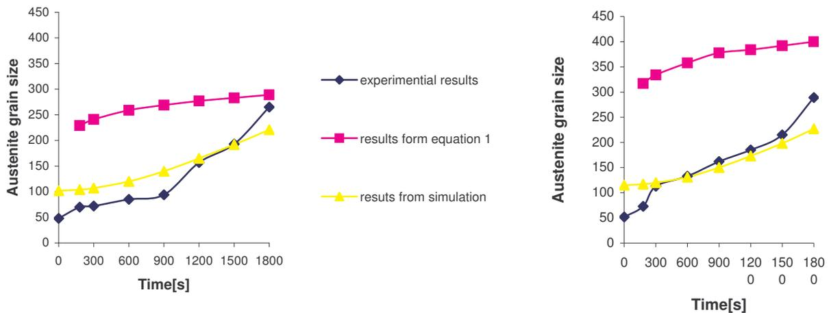
Fig. 1. The effect of soaking time on austenite grain size in isothermal conditions (a-temp. 1050°C b- temp1180°C)
