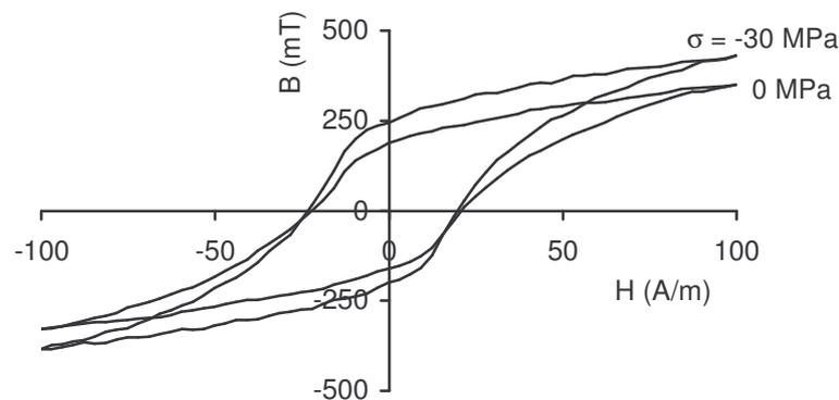
Figure 8. Influence of the mechanical, compressive stresses on hysteresis loop of the  $\text{Fe}_{85.4}\text{Hf}_{1.4}\text{B}_{13.2}$  alloy after annealing in temperature 523 K for 1 hour
