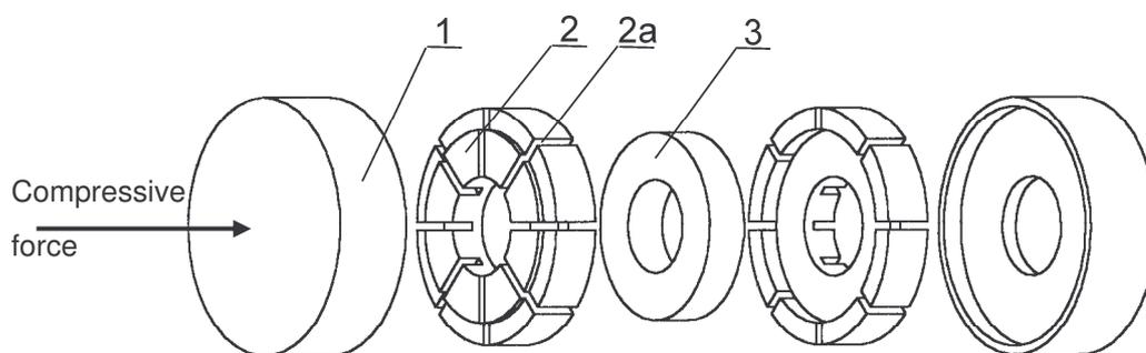
Fig. x3. Device for applying uniform, compressive stress to the ring-shape sample (patent pending P-345758) [x5] 1 – base backing, 2 – nonmagnetic, cylindrical backing 2a – grooves for the winding, 3 – sample under investigation
