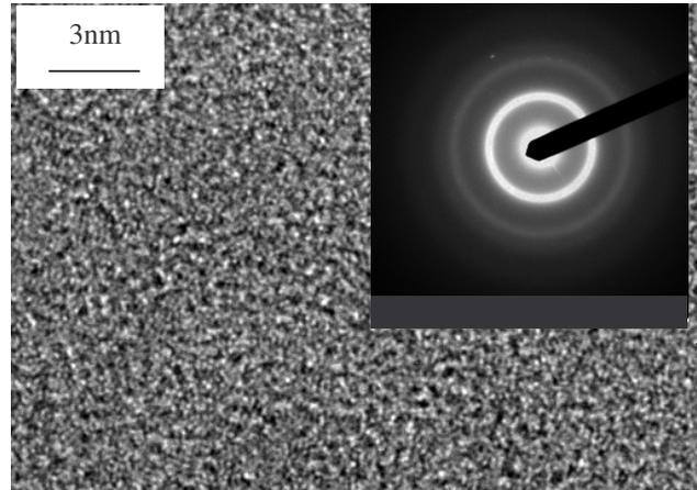
Figure 3. HRTEM micrograph for  $\text{Fe}_{85.4}\text{Hf}_{1.4}\text{B}_{13.2}$  alloy in as quenched state
