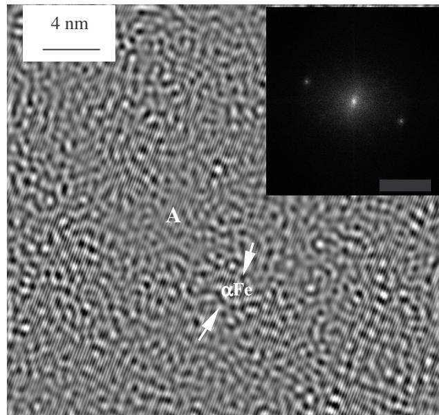
Figure 6. HRTEM micrograph for  $\text{Fe}_{85.4}\text{Hf}_{1.4}\text{B}_{13.2}$  alloy after annealing at  $T_{\text{op}}=523$  K by 1 h
