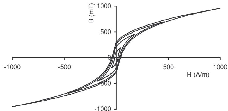
Figure 7. Family of the hysteresis loops for  $\text{Fe}_{85.4}\text{Hf}_{1.4}\text{B}_{13.2}$  alloy after annealing in temperature 523 K for 1 hour
