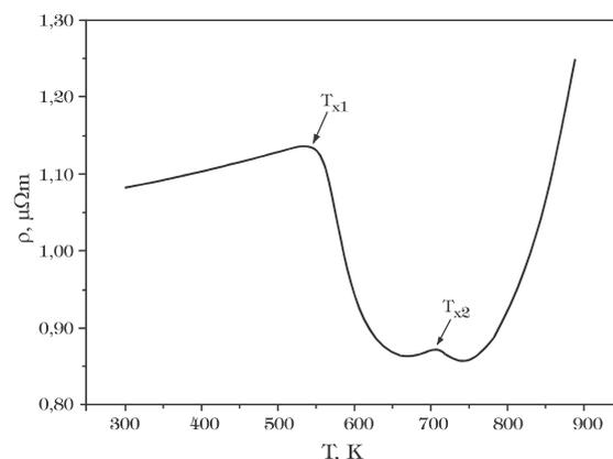
Figure 5. The isochronal resistivity curve of  $\text{Fe}_{85.4}\text{Hf}_{1.4}\text{B}_{13.2}$  alloy determined for the heating rate  $0.007 \text{ K/s}$
