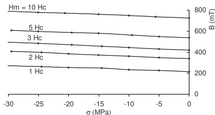
Figure 9. Changes of the flux density  $B$  in ring-shape core made of annealed  $\text{Fe}_{85.4}\text{Hf}_{1.4}\text{B}_{13.2}$  amorphous alloy, under compressive stresses  $\sigma$ , for constant value of magnetizing field  $H_m$  (value of  $H_m$  is presented as the multiplied value of coercive force  $H_c$ )
