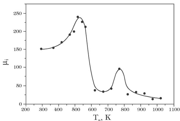
Figure 4. The initial magnetic permeability  $\mu_i$  measured at room temperature for  $\text{Fe}_{85.4}\text{Hf}_{1.4}\text{B}_{13.2}$  alloy after 1 h annealing at temperature  $T_a$
