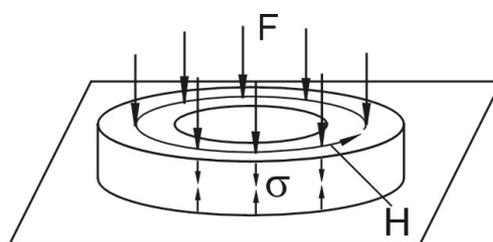
Figure 1. The general idea of applying uniform, compressive stress to the ring-shape sample
