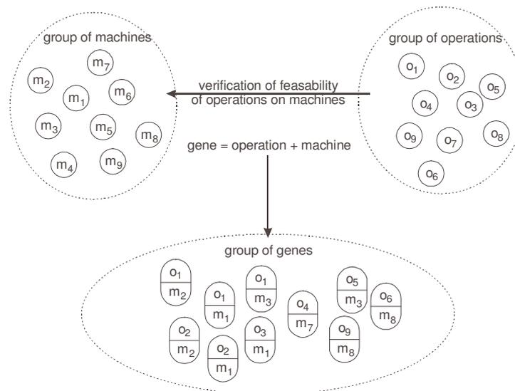
Figure 1: Representation of coding of solutions
