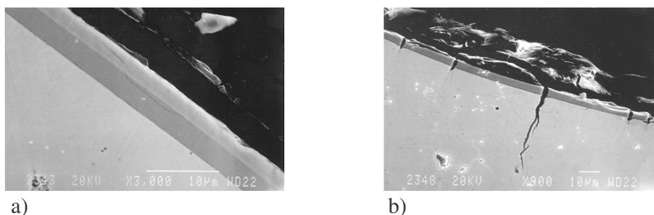
Fig. 2. Cross-sectional SEM micrographs of PVD CrN coated core after 2700 injections: a) on the opposite side of the gate; thick oxide layer (bright layer on the top), and b) on the side of the gate.
