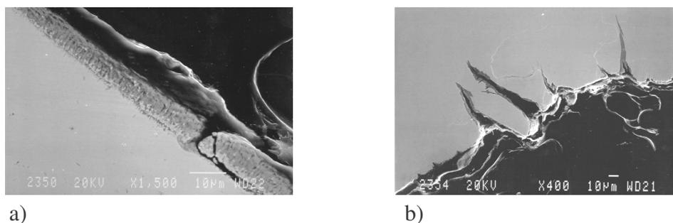
Fig. 3. Cross-sectional SEM micrographs showing of cores nitrided by Tenifer process after 2700 injections: a) on the opposite side of the gate; thick oxide layer is visible, and b) on the side of the gate.
