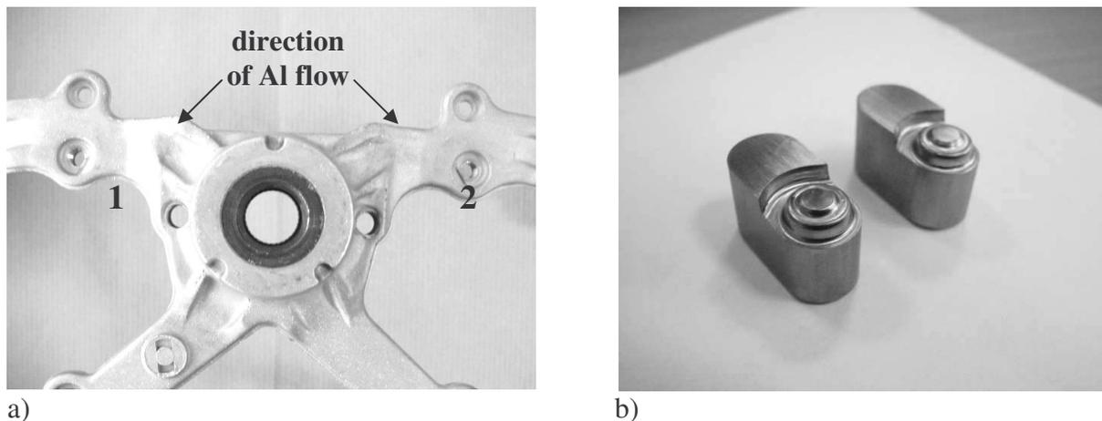
Fig. 1. Casting driving wheel (a) and the pair of PVD-coated test cores for positions 1 and 2 on the left side (b).
