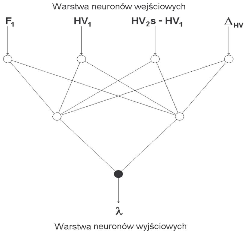
Fig.3. Pattern of neuron net used to forecast optimal rod processing degree
