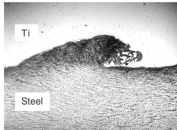
Fig. 2. Part of microstructure of steel-titanium bonding area - non-heat treated condition.
