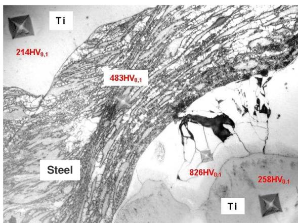
Fig. 1. Macrostructure of explosive welded joint steel-titanium-aluminium; visible points of microhardness measurements.
