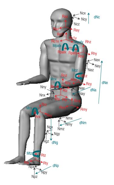
Finally there are 66 unknowns, coinciding without great value that the number of equations is 66 too, for counting 11 members and six balance equations for each one of them, of forces and torques in the three axes. The 66 unknowns are the following ones:
