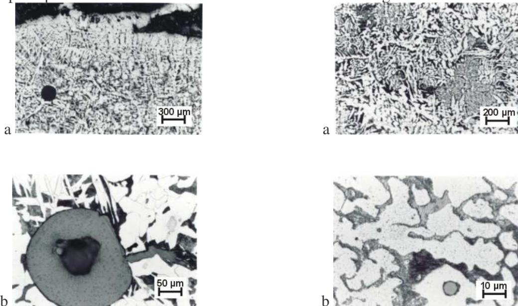
Figure 1. Microstructure of the continuously cast ingot surface layer
