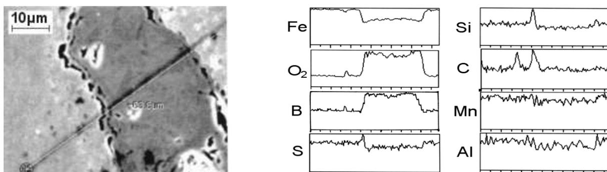
Figure 3. Spectral quality analyses of boron oxide, silicon carbides and manganese sulfides.
