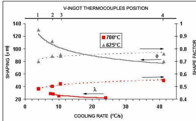
Figure 2. Shape factor and microstructural unit size ( $\lambda$  and  $\varnothing$ ) of V-shaped ingots in the as-cast condition, as a function of pouring temperature and CR
