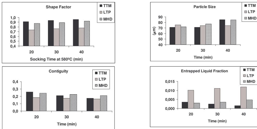
Figure 3. Microstructural features of semi-solid samples held at 580°C during 20, 30 and 40 min. Copper mould, pouring temperature and CR are equal to 615°C and 6.7°C s<sup>-1</sup>. Results are compared with those of TTM and MHD A356 semi-solid samples
