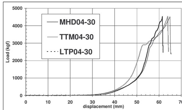
Figure 4. Rheological measurements by the back-extrusion technique: Load against displacement curves comparing LTP, MHD and TTM-conditioned samples. Partial remelting conditions are  $590^{\circ}\text{C}$  ( $f_s = 0.4$ ) and 30 min soaking time
