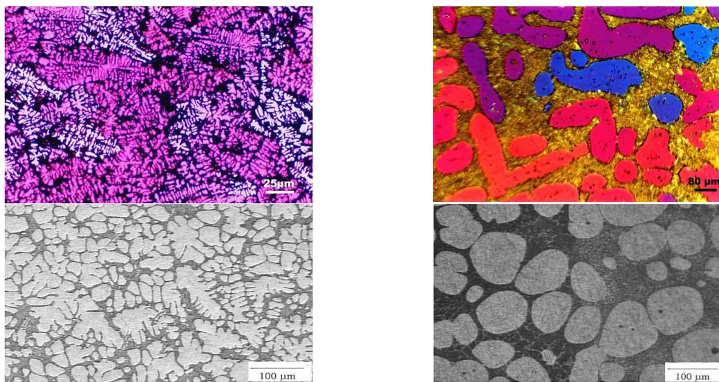
Figure 1. Microstructures of 'V'- shaped ingots poured at 700°C (a: as-cast; b: partially re-melted at 580°C/30 min) and 625°C (c: as-cast; d: partially re-melted, same conditions)
