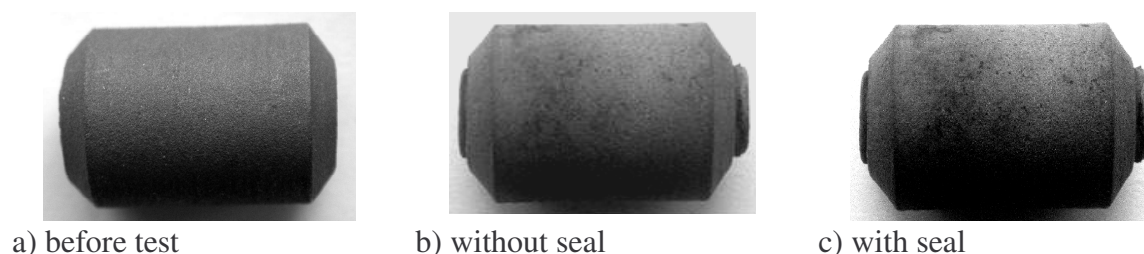
Fig. 3. The images of surface of NiAl(Cr)-Al 2 O 3 coatings: a) before oxidation test and b-c) after oxidation test
