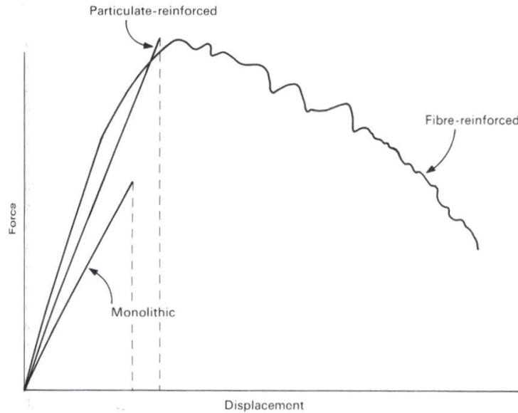
Figure 8. Schematic force-displacement curves for a monolithic ceramic and CMCs illustrating the greater energy of fracture of the CMCs [2].
