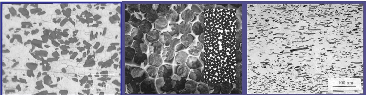
Figure 4: Long fibers, short fibers and particulate reinforcement.
