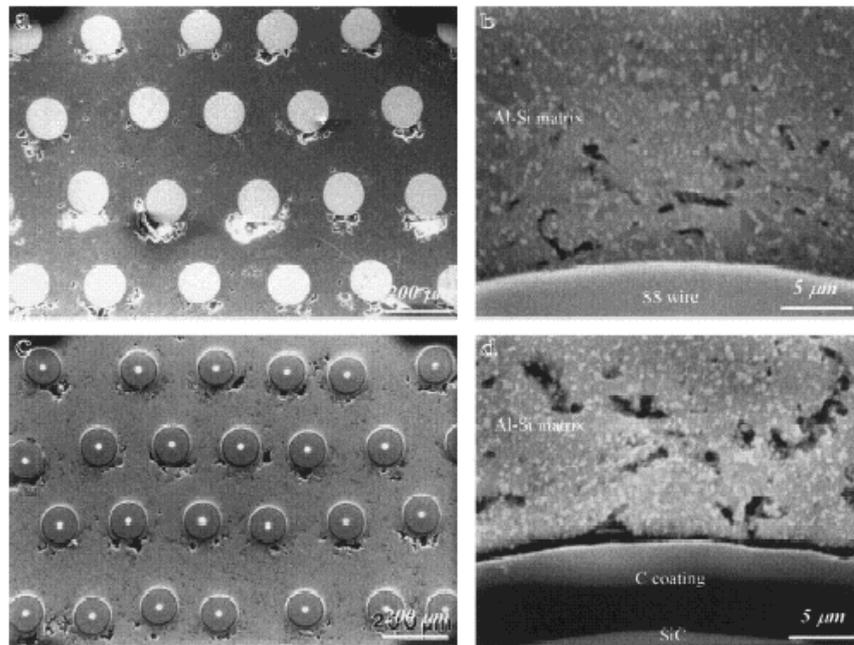
Figure 5. Spray/wind Al-12Si composites reinforced with (a) stainless wire and (c) Sigma 1140 + SiC. (b) and (d) shows the interface region of SS/Al-Si and SiC/Al-Si respectively [10].
