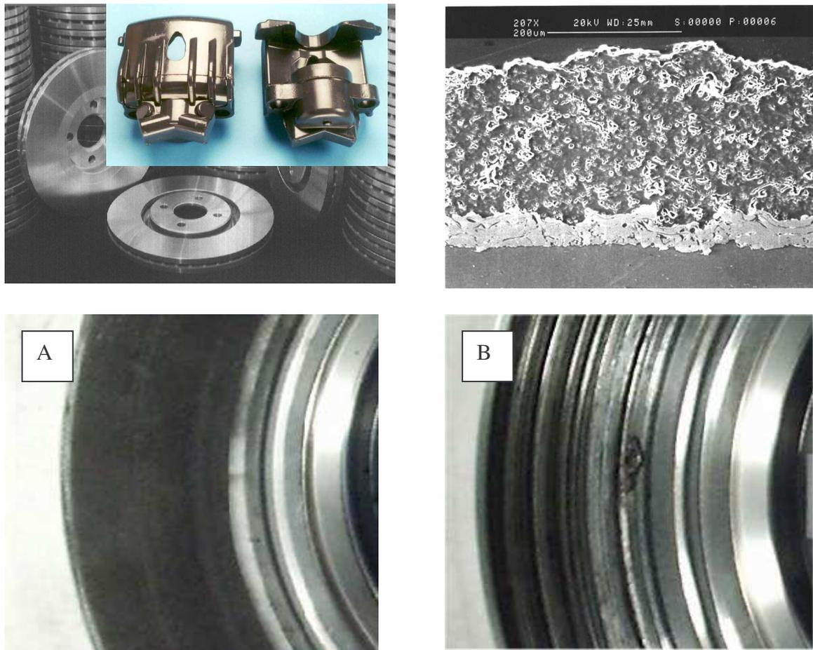
Figure 7: Brake components and coated discs; view of a ceramic coating layer. The surface appearance the coated disc (A) and of the MMC disc after the wear test at the bench.
