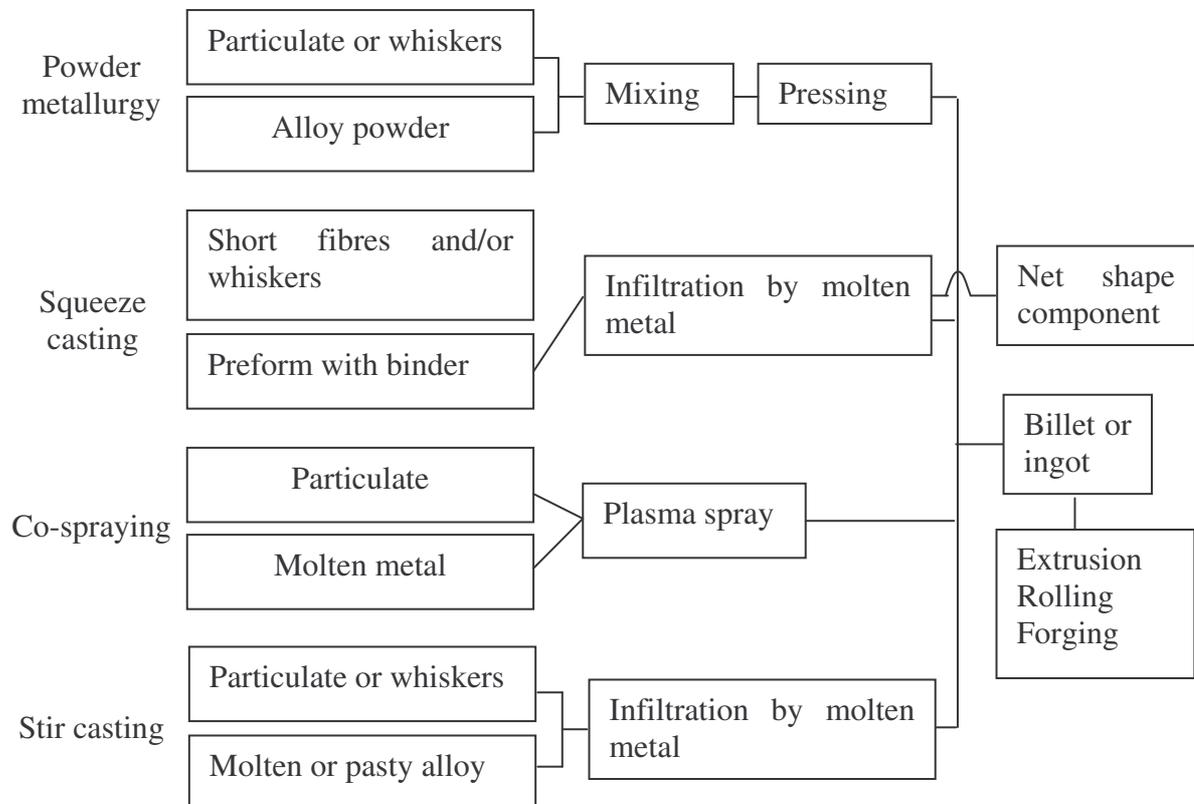
Figure 6. Discontinuous fibre, whiskers and particulate-reinforced composites process routes [8].
