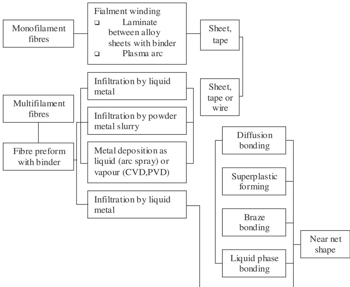
Figure 3. continuous fibre-reinforced MMCs process routes [8].
