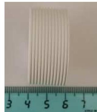
Figures 2a, 2b, 2c: Ceramic nuts and rods obtained through machining in the green state, work developed at Politecnico di Torino.
