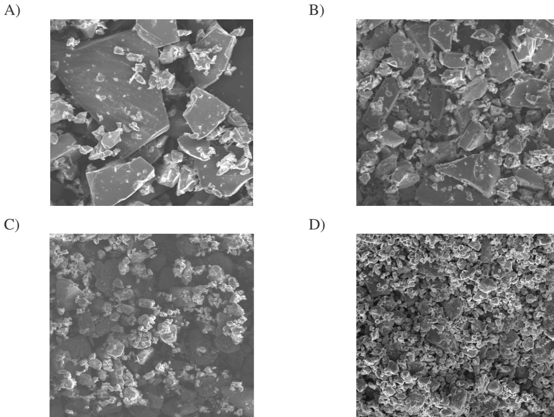
Fig. 3. Forms and sizes of the  $\text{Fe}_{73.5}\text{Cu}_1\text{Nb}_3\text{Si}_{13.5}\text{B}_9$  alloy powder particles after its thermal nanocrystallization: A) after 15 minutes of strip grinding, B) after 1 hour of strip grinding, C) after 3 hours of strip grinding, D) after 5 hours of strip grinding, magnification 500x
