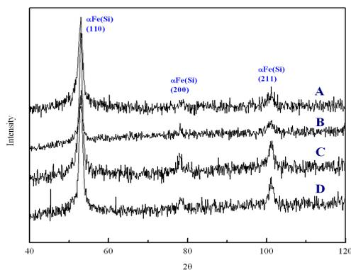
Fig. 2. X-ray diffraction patterns of the  $Fe_{73.5}Cu_1Nb_3Si_{13.5}B_9$  alloy powders:
