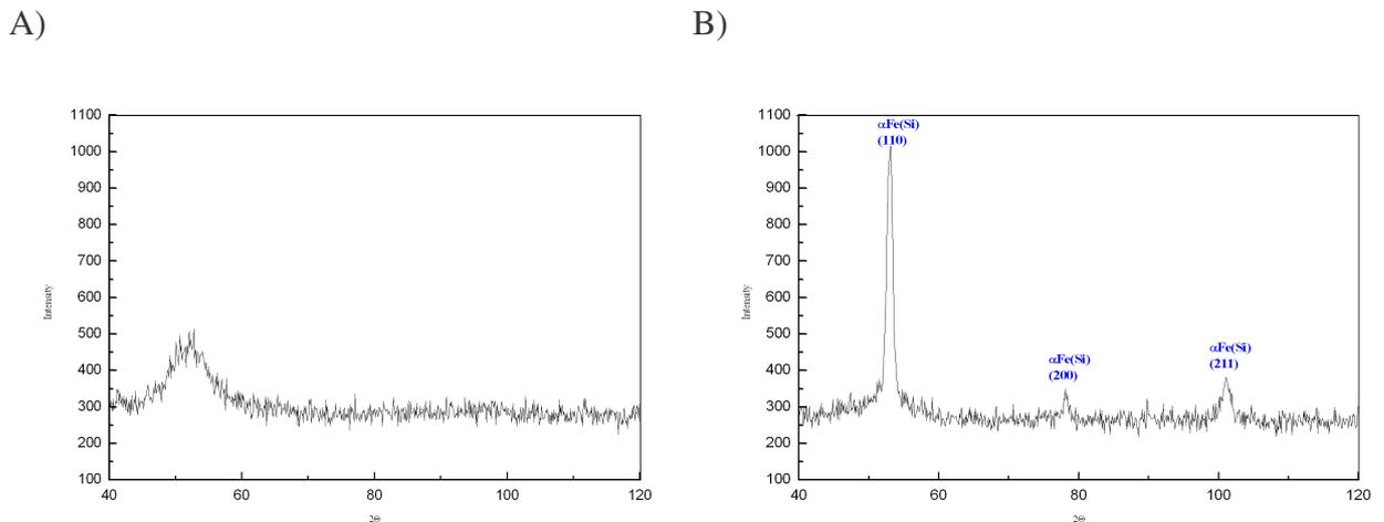
Fig. 1. X-ray diffraction patterns of the  $Fe_{73.5}Cu_1Nb_3Si_{13.5}B_9$  alloy
