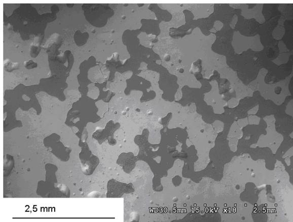
Figure 3. SEM image of surface of the ceramic-elastomer composites (S/G=0,25)
