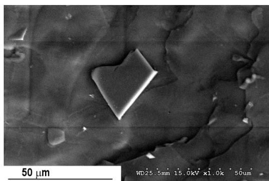
Figure 1. SEM image of the brittle fracture of the polymer with S/G equal to 0,25
