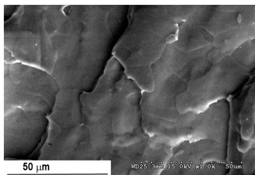
Figure 2. SEM image of the brittle fracture of the polymer with S/G equal to 1,50
