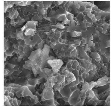
Fig. 4. Topography of composite materials fractures with the EN AC - AlSi12(Cu) matrix reinforced with the Al<sub>2</sub>O<sub>3</sub> ceramic particles, a) magnification 1000x, b) 2000x, c) 3000x
