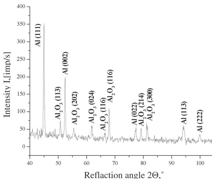
Fig. 5. X-ray diffraction pattern of the composite material with the EN AC - AlSi12(Cu) alloy matrix reinforced with the  $Al_2O_3$  particles
