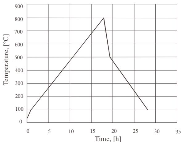
Fig. 1. Temperature versus time in the pyrolysis process
