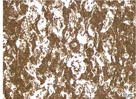
Fig. 3. Composite structure – infiltration temperature 800 °C, Al<sub>2</sub>O<sub>3</sub> phase – dark areas, Al alloy matrix – light areas
