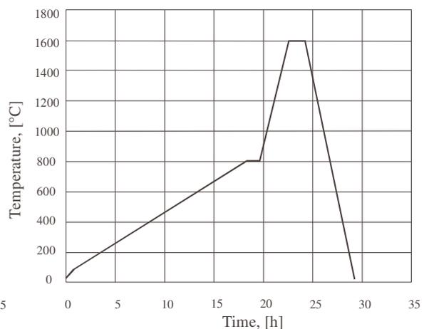
Fig. 2. Temperature versus time in the sintering process
