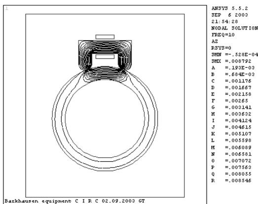
Figure 4. Flux lines. Rounded pole shoes of the yoke
