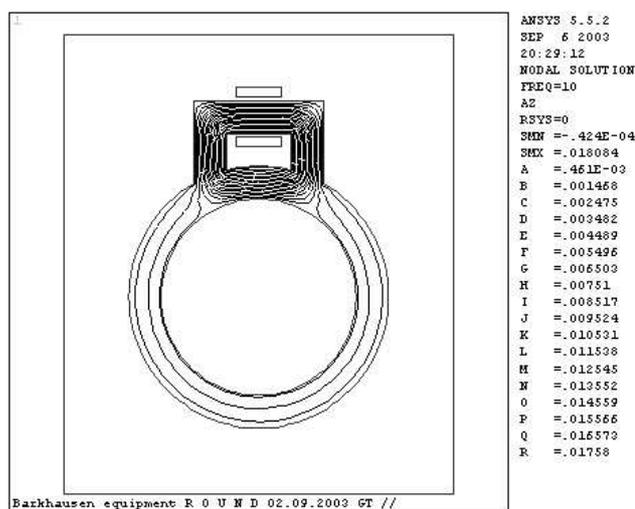
Figure 6. Flux lines. Concave profiles of shoe poles.
