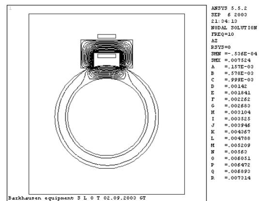
Figure 5. Flux lines. Square pole shoes of the yoke
