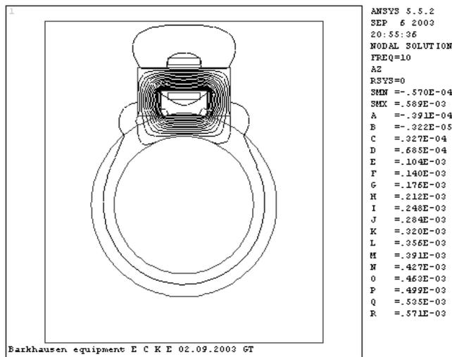
Figure 3. Flux lines. Air gap between yoke and tube
