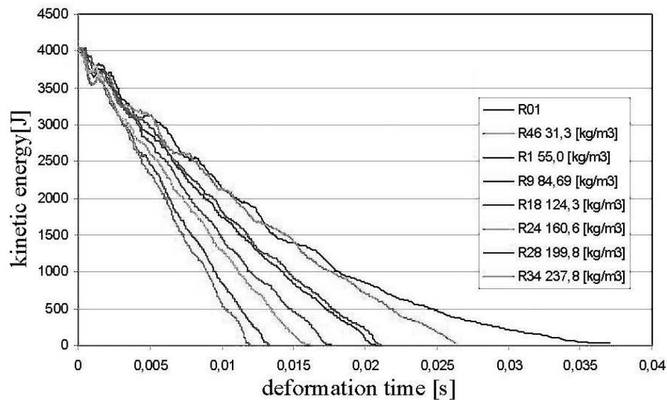
Figure 2. Relationship between kinetic energy and deformation time of round tube specimens with single wall. The symbols of the specimens contain the specimen's number and density of plastics foam.
