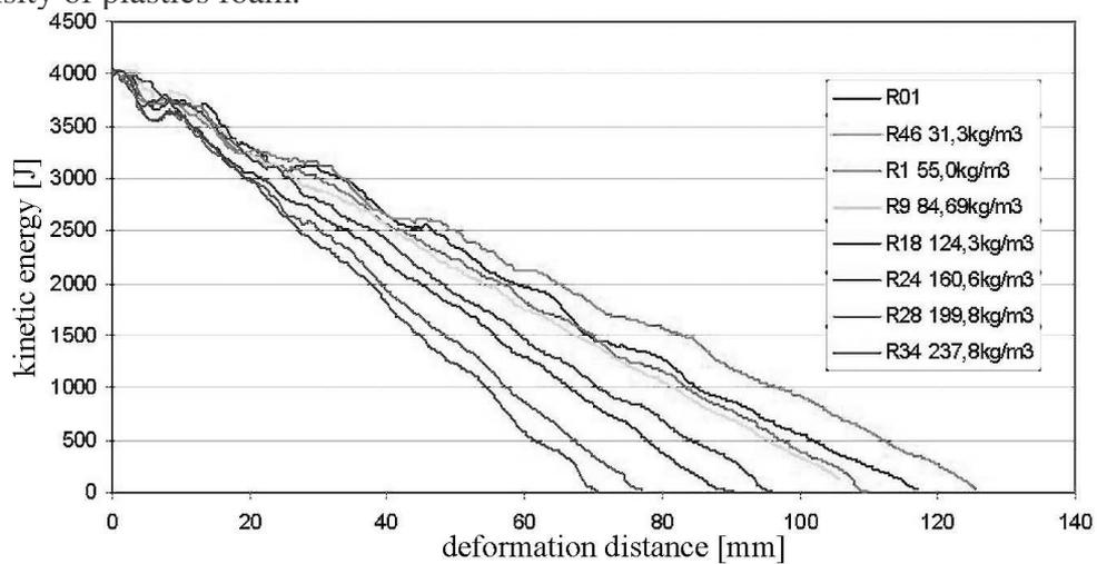
Figure 3. Relationship between kinetic energy and deformation distance of round tube specimens with single wall
