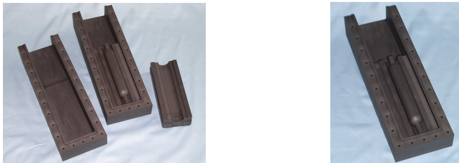
Fig. 3. Multi component mould for tubular CF-Mg-specimen
