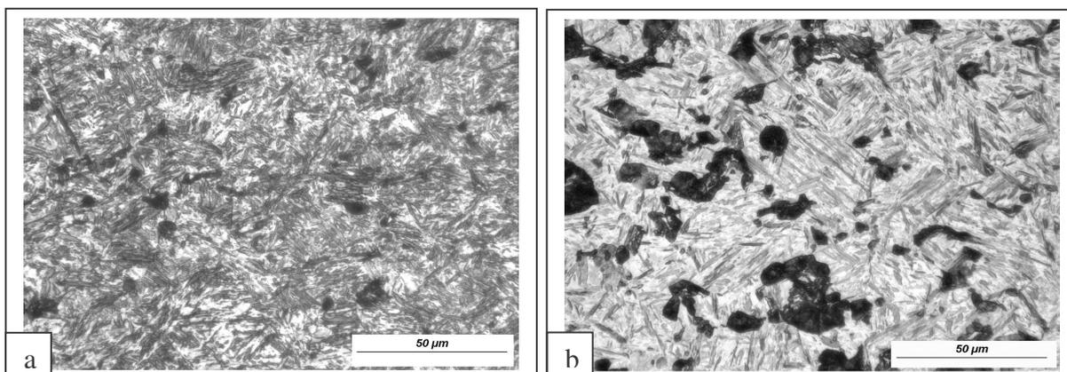
Fig. 2. Comparison of microstructure upon pulsatory and conventional forging. LM micrograph of martensitic pearlitic microstructure in the centre of specimen: (a) P8 and (b) C8
