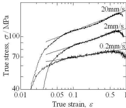
Figure 2. Relationships between stress and strain at 300°C in log-log scale
