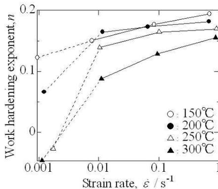
Figure 4. Relationships between work-hardening exponent,  $n$ , and strain rate
