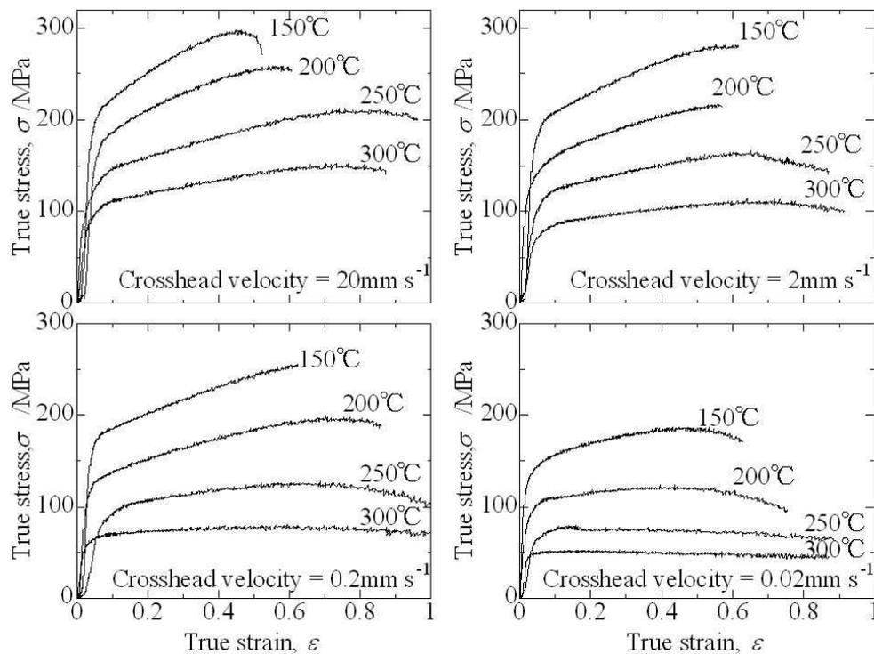
Figure 1. True stress-strain curves obtained from the tension tests
