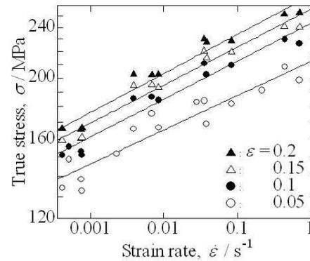
Figure 3. Relationships between stress and strain rate at 150°C in log-log scale
