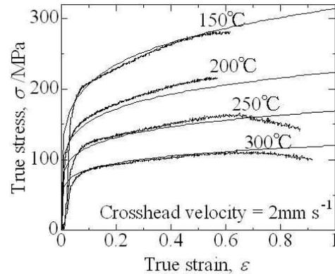
Figure 7. Comparison between calculated and measured flow curves
