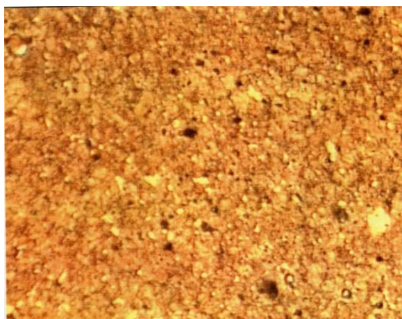
Figure 3. Morphology of surface of steel 19830 bombarded by Ti ions, mode 2, loading 2g
