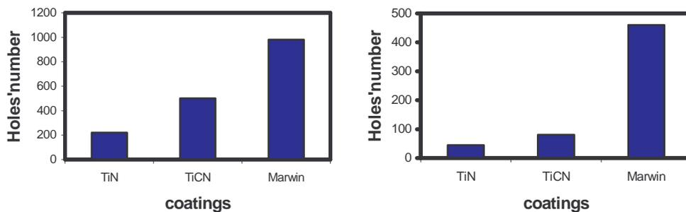
Figure 3. Results of the tapping tests under a) 25 m min<sup>-1</sup>, b) 30 m min<sup>-1</sup>.
