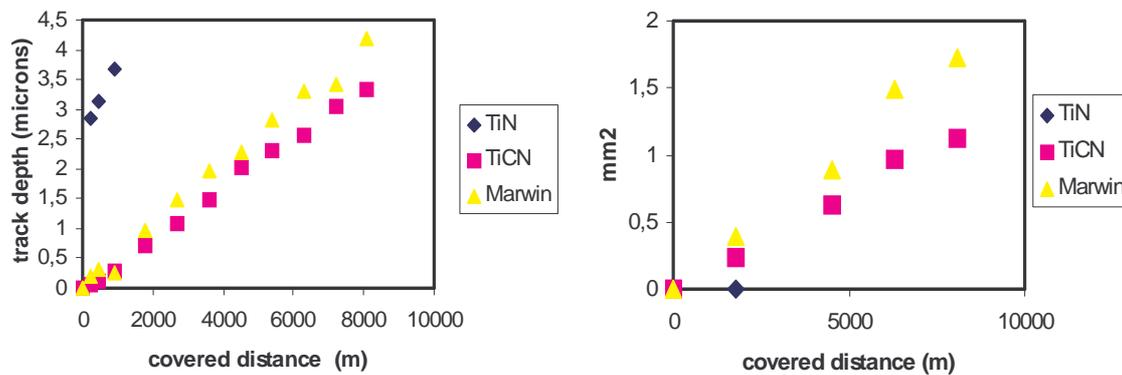
Figure 2. a) Sample track depth vs. path length; b) area on the ball vs. path length
