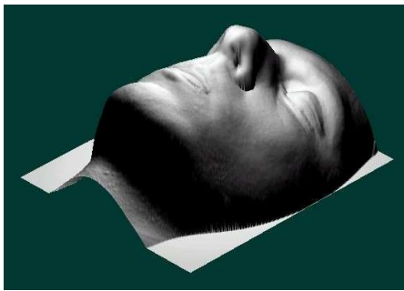
Figure 3. Captured data (“point cloud”) from the physical model of the face
