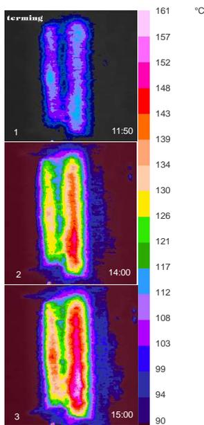
Figure 2. Working surface of the fixed part of die-casting die. Preheating process. Thermographs. At the beginning (1), after approx. 2 hours (2) and at the end (3 – initial temperature field) of the die preheating process
