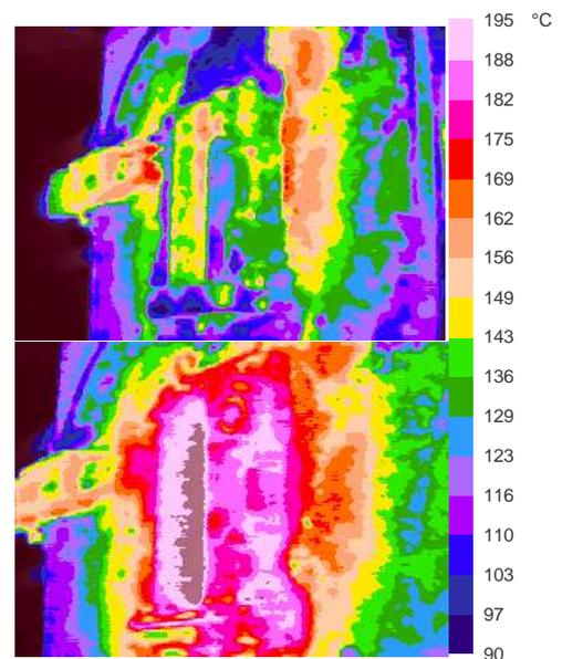
Figure 3. Working process. Thermographs. The fixed part of the die-casting die: working surface and casting (above), working surface without casting (below)
