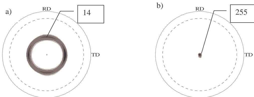
Figure 2. Pole figures registered for strip: {011} (a) and {001} (b).
