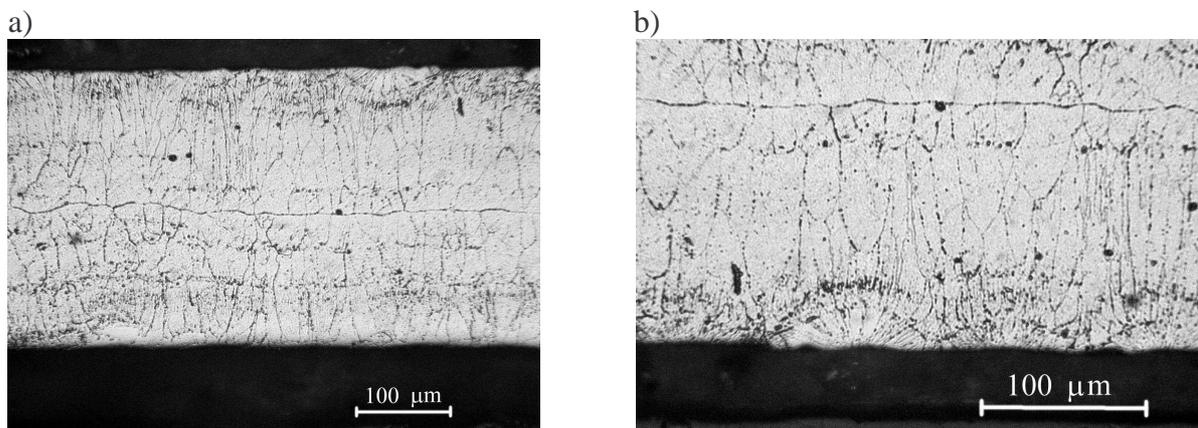
Figure 1. Microstructure of the twin roll cast strip.
