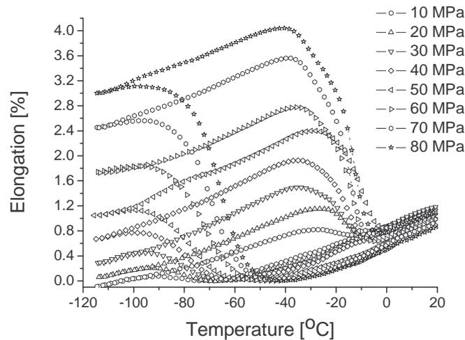
Figure 3. Shape recovery under constant tensile stress
