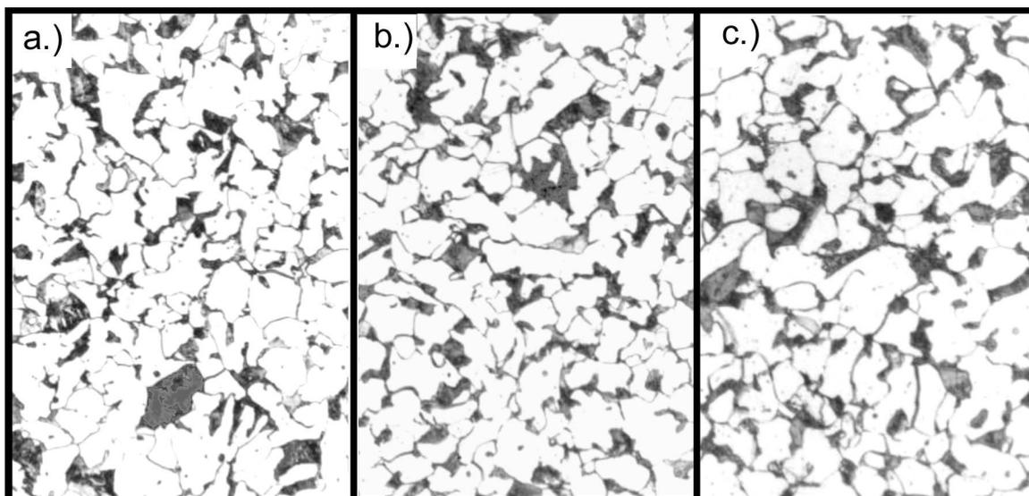
Figure 2. Microstructure of C-Mn-B steel, magn. 500x: a.) wire rod cooled in the air, dilatometric samples: b.)  $V_{8.5}=2.317$  K/s, c.)  $V_{8.5}=0.833$  K/s
