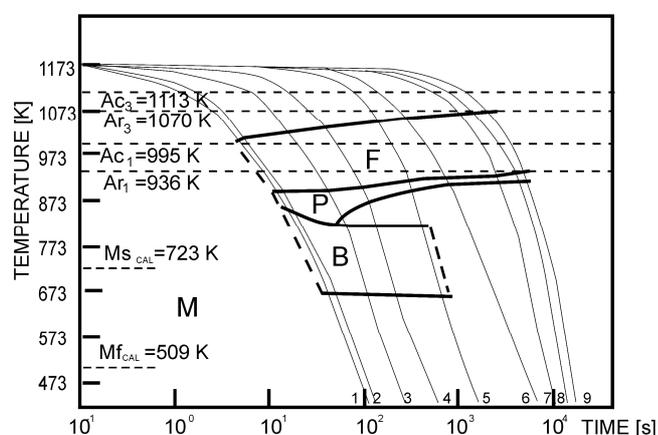
Figure 1. CCT diagram for C-Mn-B steel after austenitizing at 1163 K / 900s
