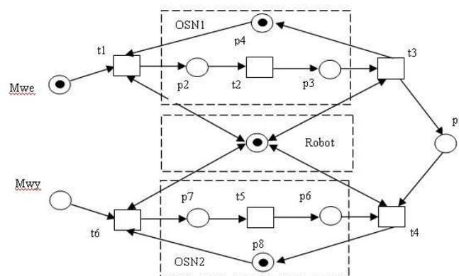
Figure 1. Serial mode network model for tending the flexible system
