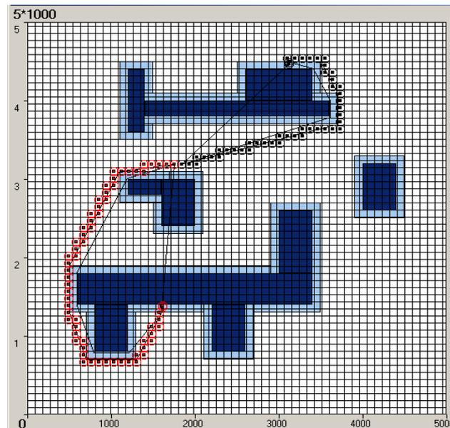
Figure 2. Generation of collision-free trajectory
