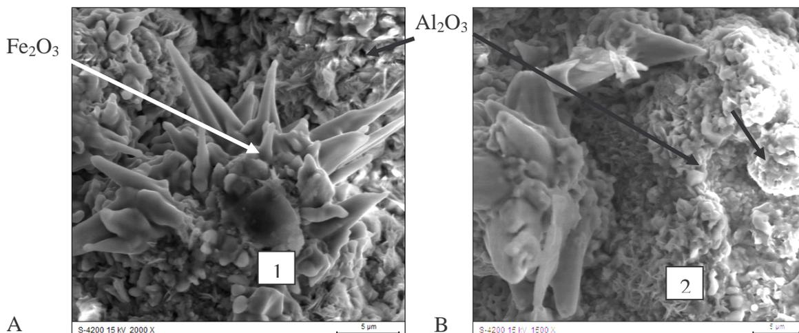
Figure 1. Morphology of corrosion products on the  $Fe_xAl_y-Al_2O_3$  coating after A) 24 h; B) 48 h oxidation test
