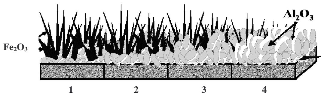
Figure 4. Oxidation model of the FeAl-Al<sub>2</sub>O<sub>3</sub> coating during 1) 12h; 2) 24 h; 3)48 h; 4) 500h corrosion test
