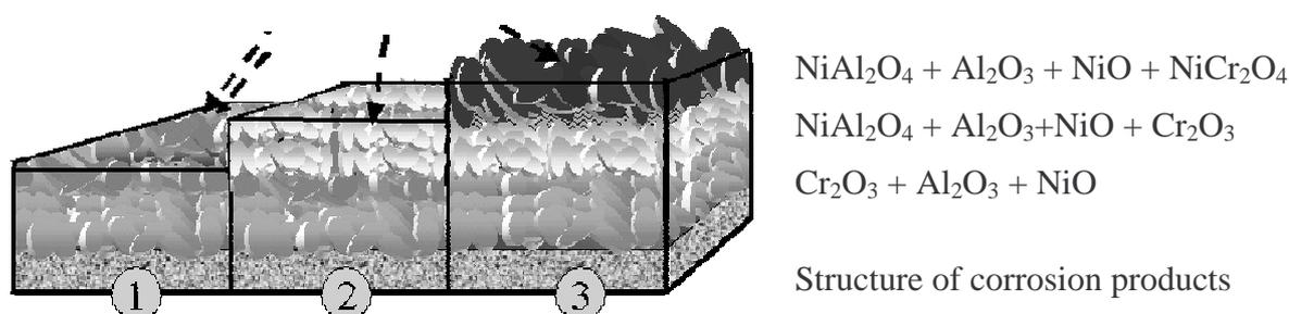
Figure 3. Oxidation model of the NiAl(Cr)-Al<sub>2</sub>O<sub>3</sub> coating during 1) -24 h; 2) - 48h; 3) 500 h corrosion test.
