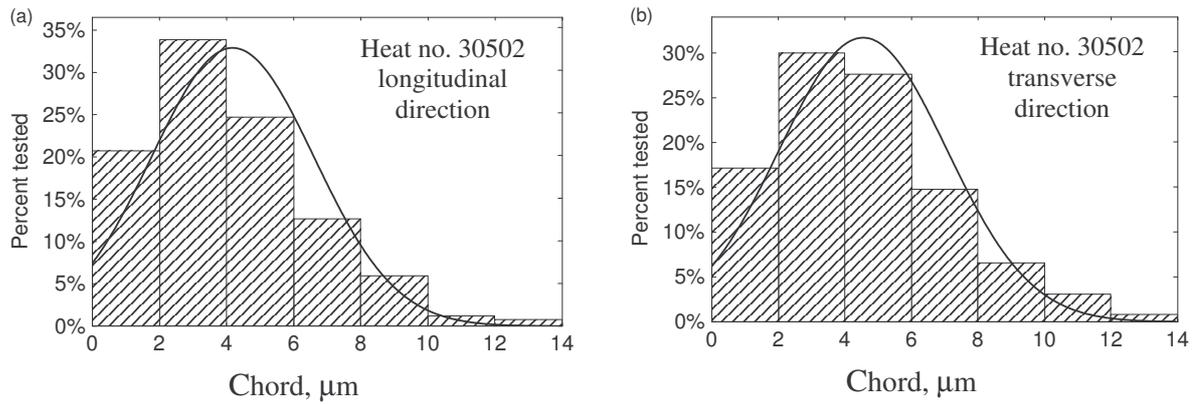
Figure 3 The distribution of average chord of ferrite grain, longitudinal (a) and transverse (b) direction, heat no. 30502
