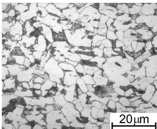
Figure 1. The ferritic-pearlitic microstructure of wire rod, longitudinal direction, no. of heat 30503
