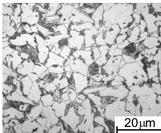
Figure 2. The ferritic-pearlitic microstructure of wire rod, transverse direction, no. of heat 30503
