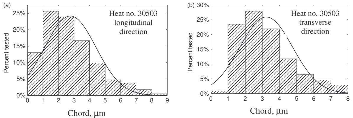
Figure 4. The distribution of average chord of pearlite grain, longitudinal (a) and transverse (b) direction, heat no. 30503
