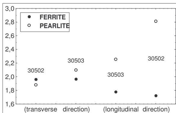
Figure 5. The changeability coefficient of the ferrite and pearlite grains in dependence of the type of the cross-section
