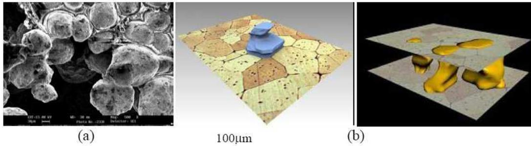
Figure 4. Thixocast structures: (a) A356 alloy from which the secondary phase was partially dissolved; (b) simulation of thixocast structure of A5052 alloy using images of parallel plans.
