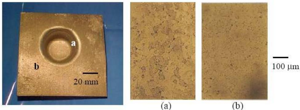
Figure 2. Typical test part of A5052 produced by drawing in the semi-solid state (635°C), a sheet with 4.0mm thickness. Microstructures in two different regions as indicated
