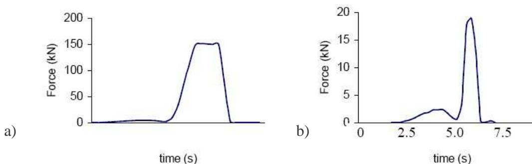
Figure 3. Forces x time during drawing of A5052 thick sheets in solid and semi-solid state, at temperatures of (a) 500 and (b) 630°C, respectively. 3.2. Microstructures of thixocast material
