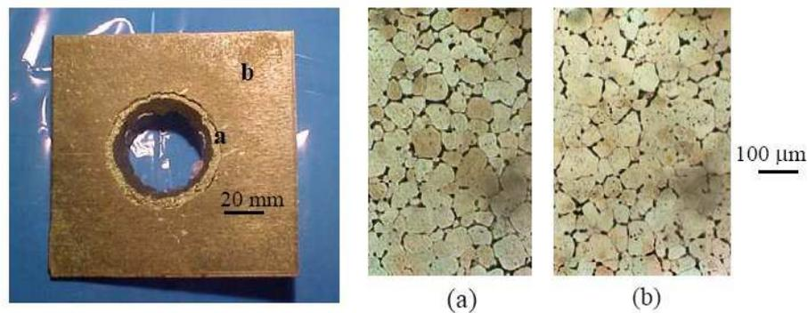
Figure 1. Typical test part of A5052 produced by drawing in the semi-solid state (640°C), a sheet with 4.0mm thickness. Microstructures in two different regions as indicated.
