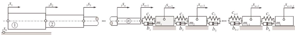
Figure 1. The discussed discrete-continuous model of a longitudinally vibrating system
