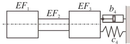
Figure 3. Geometric structural form of the synthesised discrete-continuous system with damping
