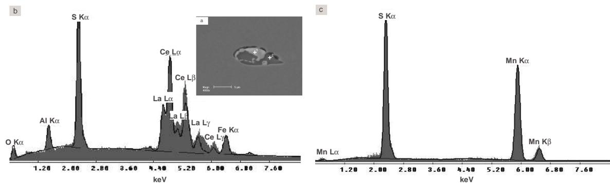
Figure 3. The (Ce, La)S sulphide with an oxide of chemical composition nearby (Al, Ce, La)<sub>2</sub>O<sub>3</sub>; a – view of the inclusion, b – spectrum of the non-metallic inclusion from a point no 1, c – spectrum of the non-metallic inclusion from a point no 2
