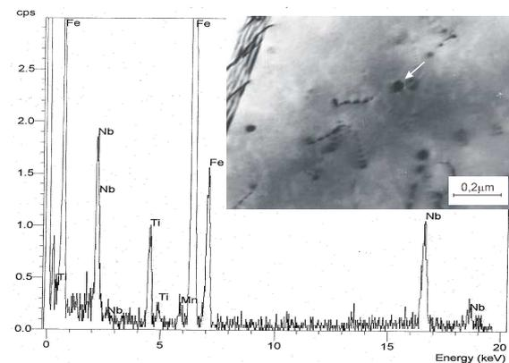
Figure 7. Dispersed particles of MX-type phases; a marked particle of the chemical composition nearby  $(\text{Nb}_{0.65}\text{Ti}_{0.35})(\text{C},\text{N})$
