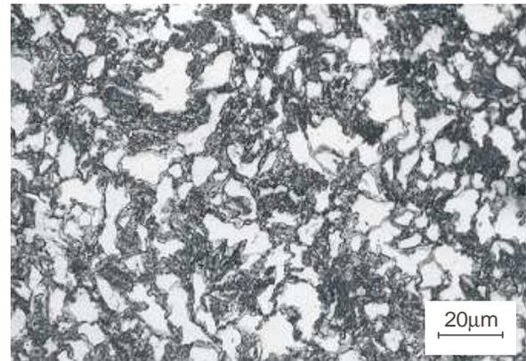
Figure 5. Ferritic – martensitic structure of the underhardened sheet
