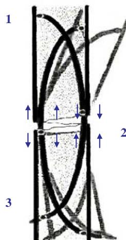
Figure 1. Axial forces ensuring the strain in the fracture gap [1]
