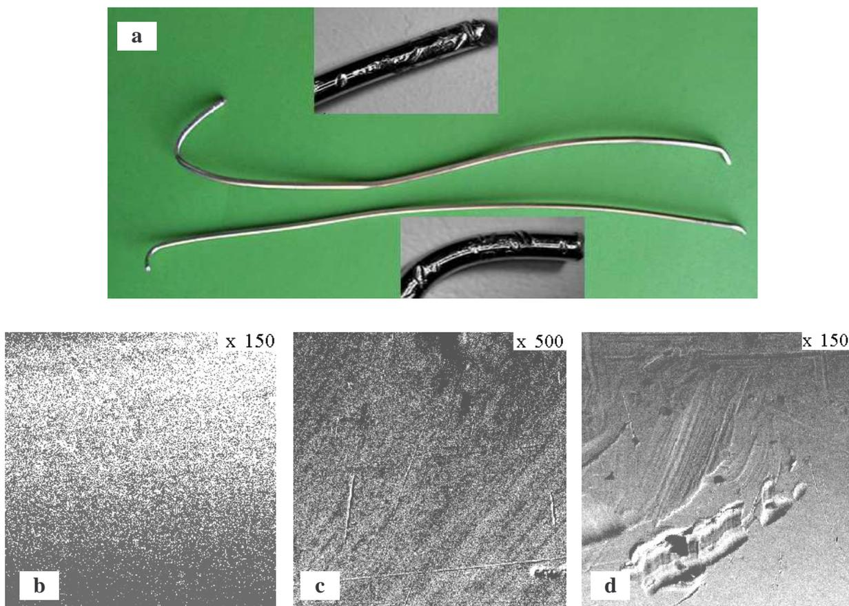
Figure 2. Example of the intramedullary nails surface: a – nails after implantations, b – initial state surface, c – after implantation – middle part, d – after implantation – end of the nail
