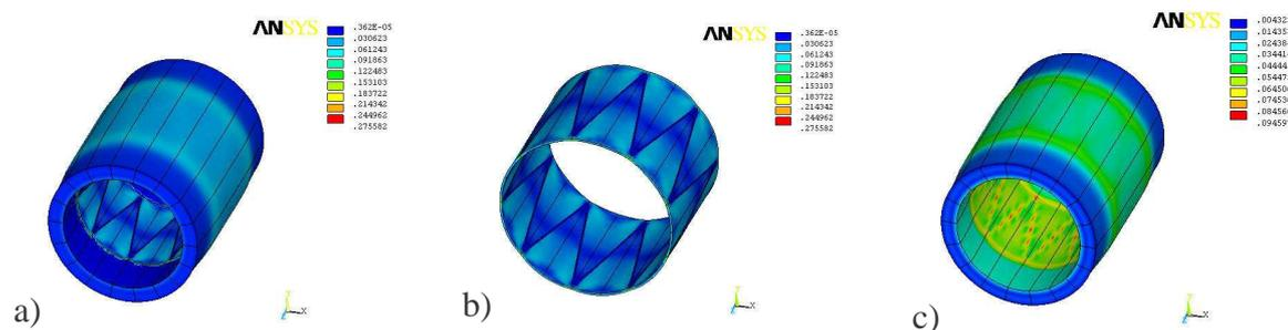
Figure 5. Strains distribution [x100%] during the work of the system: a) the stent – oesophagus system, b) the stent, c) the oesophagus
