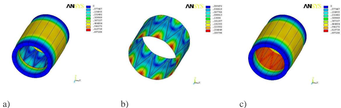
Figure 3. Radial displacements [mm] during the work of the system: a) the stent – oesophagus system, b) the stent, c) the oesophagus
