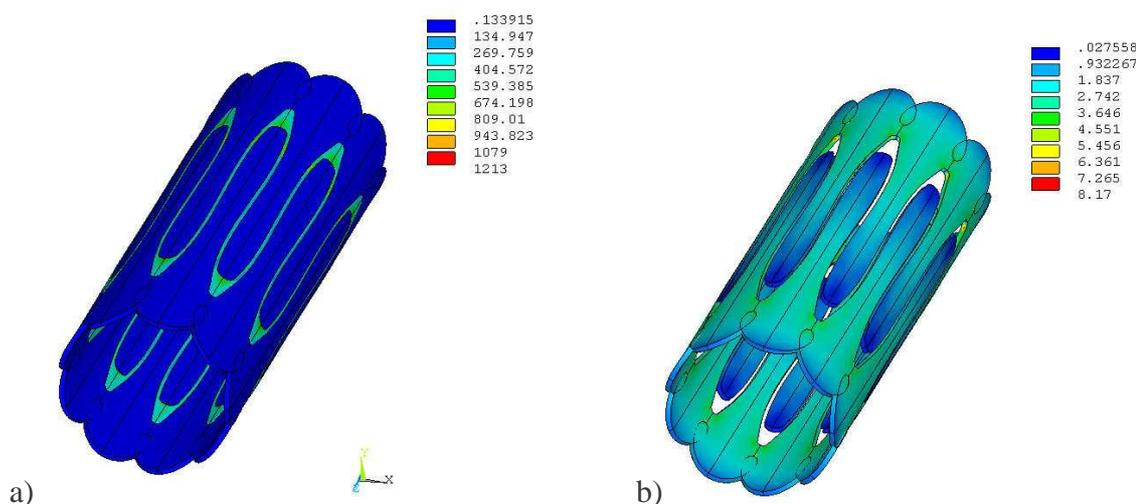
Figure 1. Stresses distribution in the esophageal stent [MPa], the radial displacement – 7,5 mm: a) the stent, b) the plastic layer
