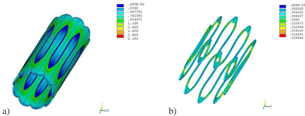
Figure 2. Stresses distribution in the esophageal stent [MPa], the radial displacement – 7,5 mm: a) the stent, b) the plastic layer
