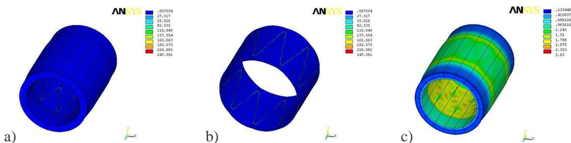
Figure 4. Stresses distribution [MPa] during the work of the system: a) the stent – oesophagus system, b) the stent, c) the oesophagus
