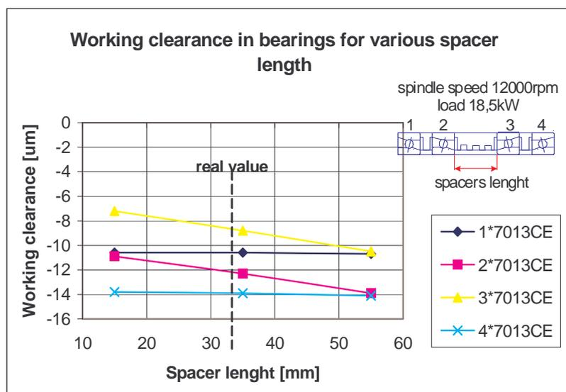
Figure 2. Running clearance in bearings versus spacer length
