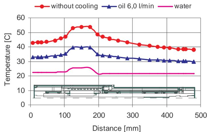
Figure 3. Effect of stator cooling conditions on temperature of the electrospindle
