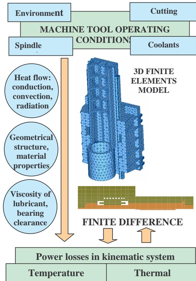
Figure 1. Schematic of hybrid model of machining centre headstock
