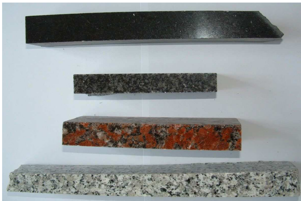
Figure 1. Four types of granite on which the tests have been performed, from the top: black granite (Zimbabwe), impala african, red granite and the grey one on the bottom.
