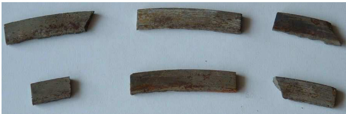
Figure 3. Broken and lost segments of the saw number 4a.
