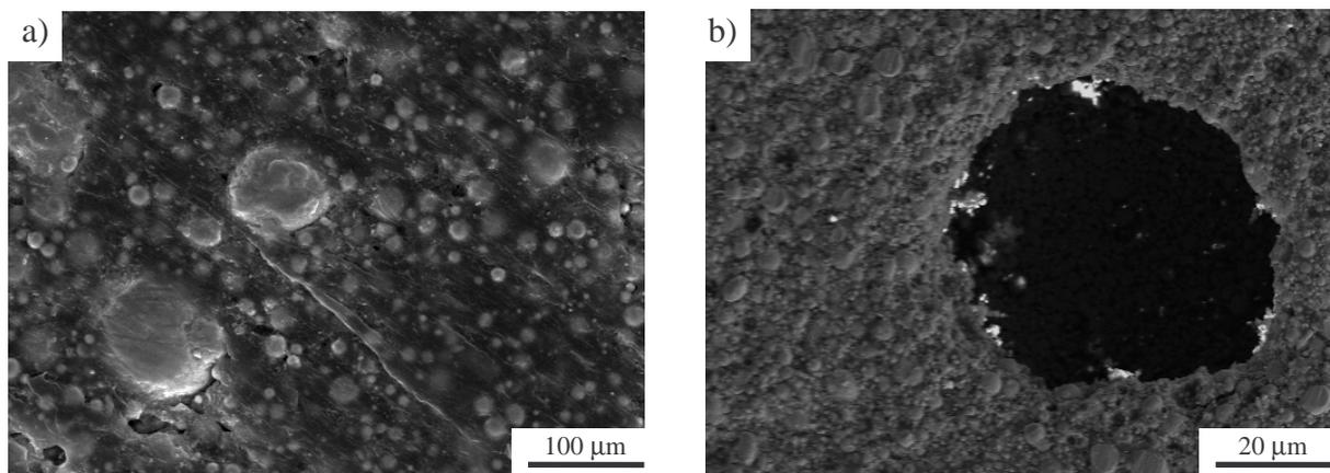
Fig. 1. a) Spherical pore in HS12-1-5-5 HSS formed with the pressureless forming method, b) distribution of binder and powder of HS12-1-5-5 HSS formed with the PIM method
