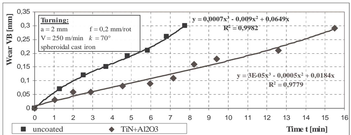
Figure 3. Comparison of the approximated values of the VB wear of the  $Al_2O_3+SiC_{(w)}$  based ceramics: uncoated and coated with the CVD  $TiN+Al_2O_3$  coating, depending on machining time
