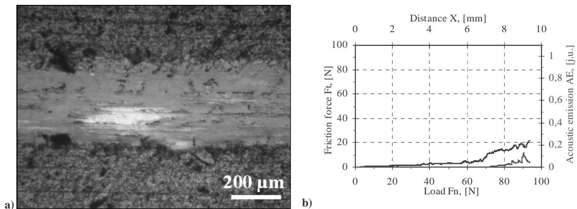
Figure 1. a) Indenter trace with the optical  $L_c$  load, b) scratch test results of the TiN+TiAlSiN+TiN coating surface deposited on  $Al_2O_3+SiC_{(w)}$  substrate
