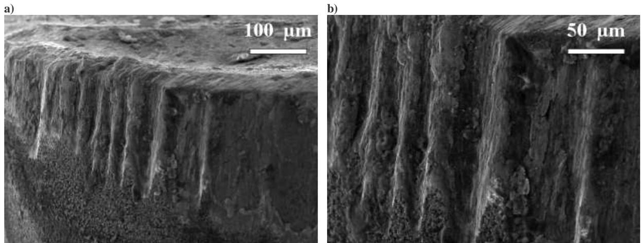
Figure 2. a) Character of wear of the  $Al_2O_3+SiC_{(w)}$  sample with  $TiN+Al_2O_3$  coating, investigated with SEM after cutting test, b) the detail of Figure a)
