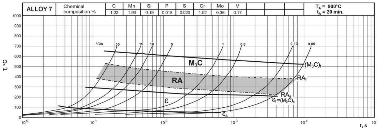
Figure 2. CHT diagram of the researched steel
