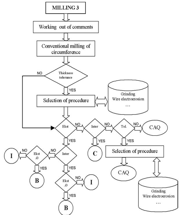
Fig. 1. Basic algorithm for milling – case A
