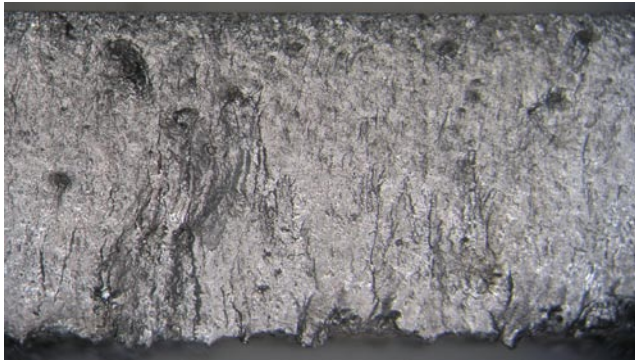
Fig.3. Typical example of cut edge of the 8 mm thick AlSi-alloy/SiC p 15vol.% composite specimen cutting with laser; cutting parameters: average power of CO 2 laser P=4 kW, pulse repetition rate f =10 kHz, nitrogen jet assistance gas pressure 16 bar, nozzle-material standoff distance 2 mm.
