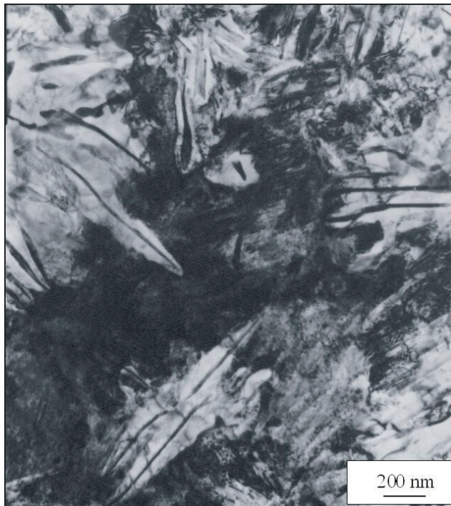
Fig. 5. TEM micrograph of thin foil made from the central part of specimen strained at 650°C after isothermal decomposition at 350°C for 70s
