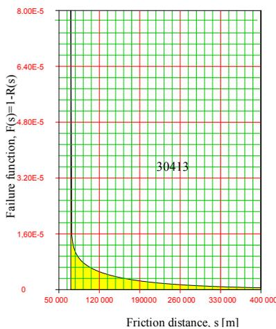
Fig. 4. The chart for probability density function  $f(s)$  as a function of friction distance for sealings type Mupuseal 30412 – 0450 – 90 – S (a) and 30413 – 0450 – 90 – S (b)
