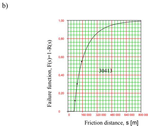
Fig. 2. Failure function  $F(s)$  chart as a function of friction distance for sealings Mupuseal 30412 – 0450 – 90 – S (a) and 30413 – 0450 – 90 – S (b)
