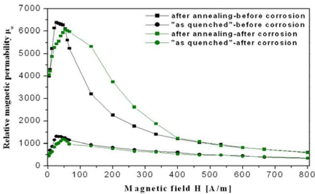
Fig. 4. Relative magnetic permeability  $\mu_w$  for alloy  $Fe_{33.5}Co_{40}Cu_1Nb_3Si_{13.5}B_9$  in function magnetic field for samples after annealing, before and after exposure in one molar solution  $Na_2SO_4$
