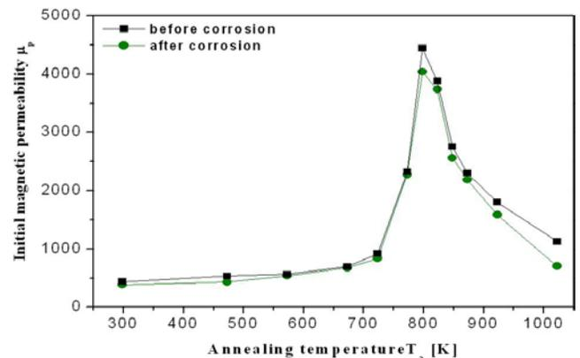
Fig. 3. Initial magnetic permeability  $\mu_p$  for  $\text{Fe}_{33.5}\text{Co}_{40}\text{Cu}_1\text{Nb}_3\text{Si}_{13.5}\text{B}_9$  alloy as function of temperature in field 0.5 A/m, after exposure in one molar solution  $\text{Na}_2\text{SO}_4$  and without it
