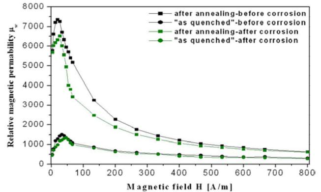
Fig. 2. Relative magnetic permeability  $\mu_w$   $\text{Fe}_{63.5}\text{Co}_{10}\text{Cu}_1\text{Nb}_3\text{Si}_{13.5}\text{B}_9$  alloy as function of magnetic field for samples after annealing, before and after exposure in one molar solution  $\text{Na}_2\text{SO}_4$
