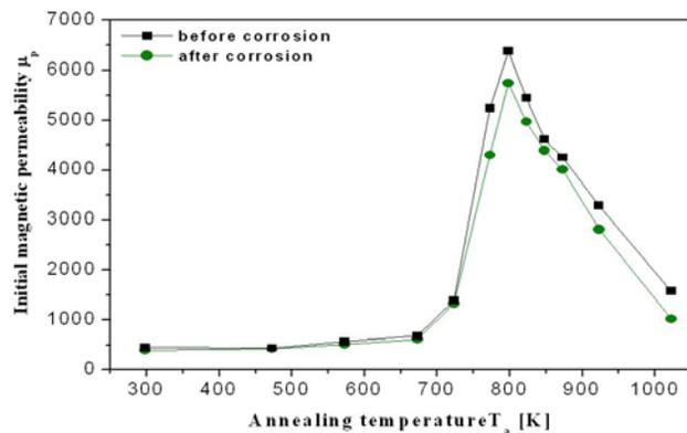
Fig. 1. Initial magnetic permeability  $\mu_p$  for  $\text{Fe}_{63.5}\text{Co}_{10}\text{Cu}_1\text{Nb}_3\text{Si}_{13.5}\text{B}_9$  alloy as function of temperature in field 0.5 A/m, after exposure in one molar solution  $\text{Na}_2\text{SO}_4$  and without it
