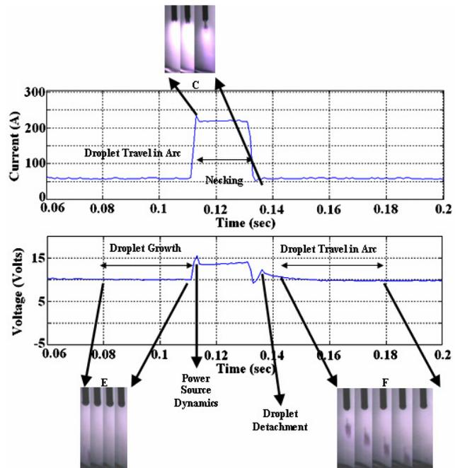
Fig. 4. Synchronized images of high speed camera pictures with arc current and voltage waveform for ODPP
