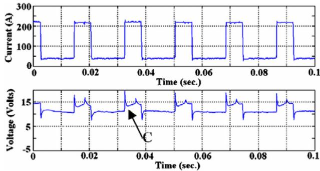
Fig. 3. Typical welding current (top) and voltage (bottom) as functions of time for ODPP drop transfer mode
