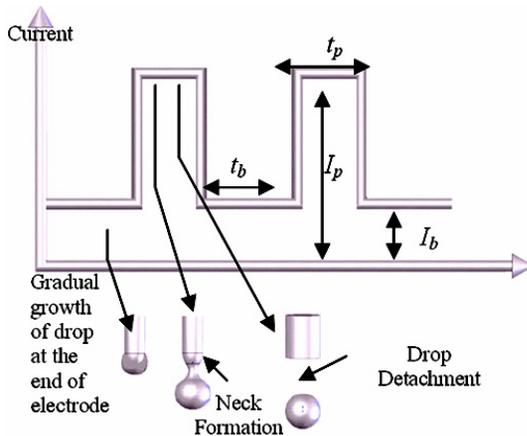
Fig. 1. Parameters of pulsed current waveform
