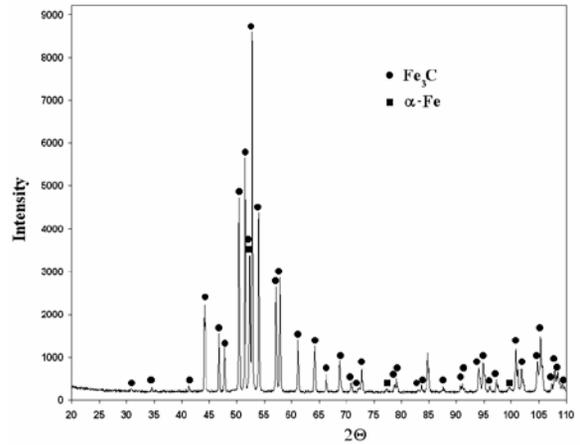
Fig. 4. The X-ray diffraction patterns of Fe-6,67% mass C powder after mechanical alloying (150 h) and pulse-plasma sintering
