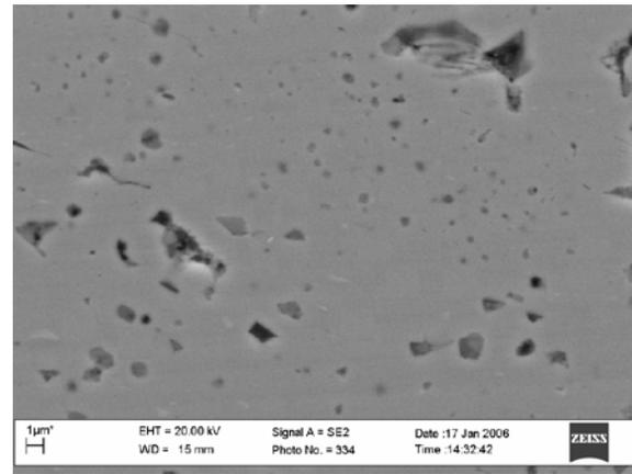
Fig. 8. Image of the voids of the sintered Fe-6,67% mass C powder obtained by 150h of MA and sintering (magn. 10000x)
