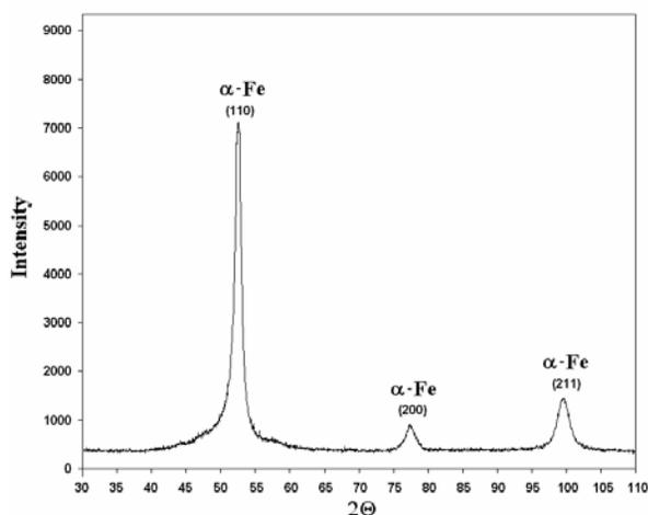
Fig. 1. The X-ray diffraction patterns of Fe-6,67% mass C powder alloy vs. the grinding time 25 hours
