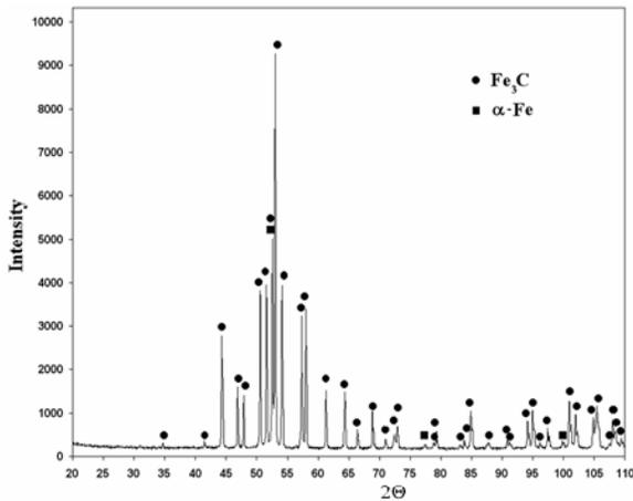
Fig. 3. The X-ray diffraction patterns of the Fe-6,67% mass C powder after mechanical alloying (25 h) and pulse-plasma sintering
