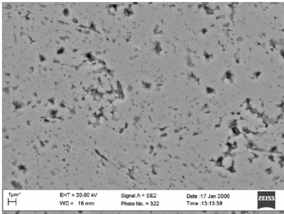
Fig. 7. Image of the voids of the sintered Fe-6,67% mass C powder obtained by 25h of MA and sintering (magn. 10000x)
