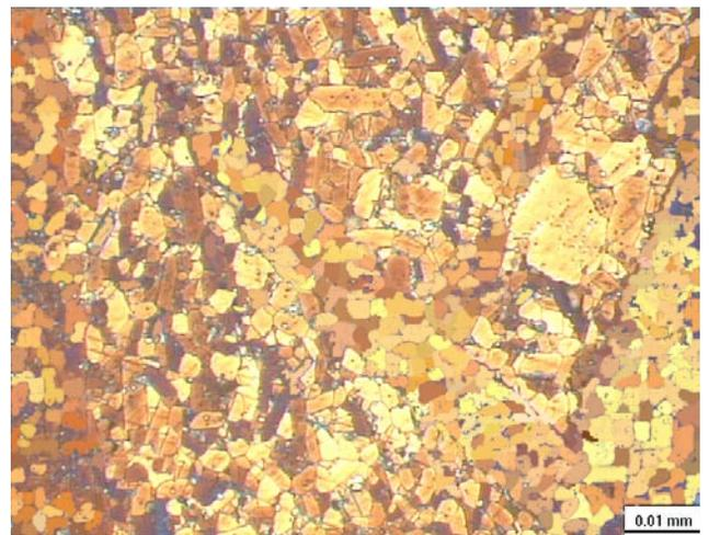
Fig. 6. Image of the microstructure of the sintered Fe-6,67% mass C powder obtained by 150h of MA and sintering (magn. 1000x)
