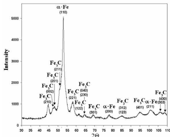
Fig. 2. The X-ray diffraction patterns of Fe-6,67% mass C powder alloy vs. the grinding time 150 hours
