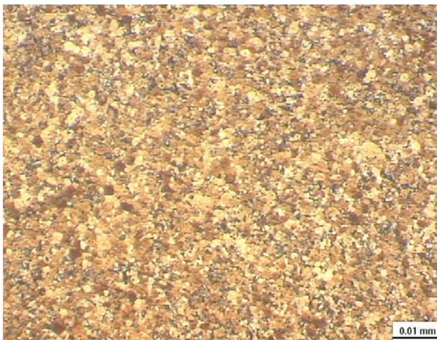
Fig. 5. Image of the microstructure of the sintered Fe-6,67% mass C powder obtained by 25h of MA and sintering (magn. 1000x)
