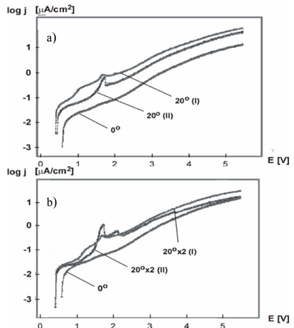
Fig. 5. Anodic polarization curves for tensile (I) and compressive (II) zones on the surface of the Ti6Al4V alloy anodized samples: a) after bending, b) after rebending (angle 20°); curves for non-deformed sample included for comparison
