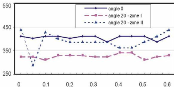
Fig. 4. Distribution of microhardness values along perimeter sample in zone (I) and (II) for bent and non-deformed samples (bending angle 20°)
