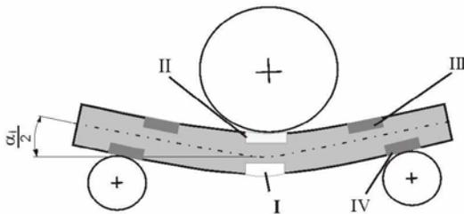
Fig.1. Zones of surface stress due to bending: (I)-max tensile, (II)-max compressive and cold working, (III)-compressive, (IV)-tensile and cold working stresses [1]
