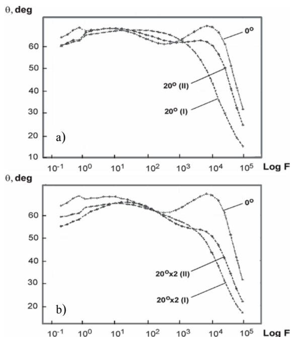
Fig. 6. Impedance spectra for the tensile (I) and compressive (II) zones of the Ti6Al4V alloy sample: a) bending, b) rebending
