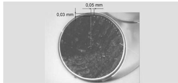
Fig. 2. Microhardness measurement points on cross section of the samples
