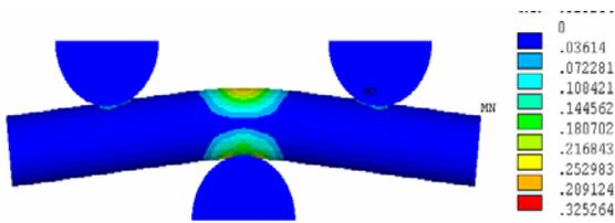
Fig. 3. Strain distribution in rod made of Ti6Al4V (bending angle 20°) Von Mises
