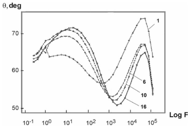
Fig. 3. Impedance spectra (Bode'a diagram) for anodized Ti6Al4V alloy non-deformed specimens recorded during immersion in Ringer's solution, temp. 298 K
