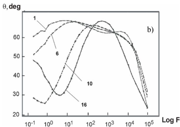
Fig. 4. Impedance spectra for a) the tensile (I) and b) compressive (II) zones of the Ti6Al4V alloy sample; bending angle 20°
