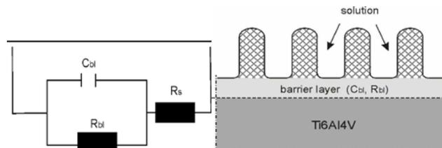
Fig. 1. Equivalent circuit and model of surface layer on the Ti6Al4V alloy [12, 16]
