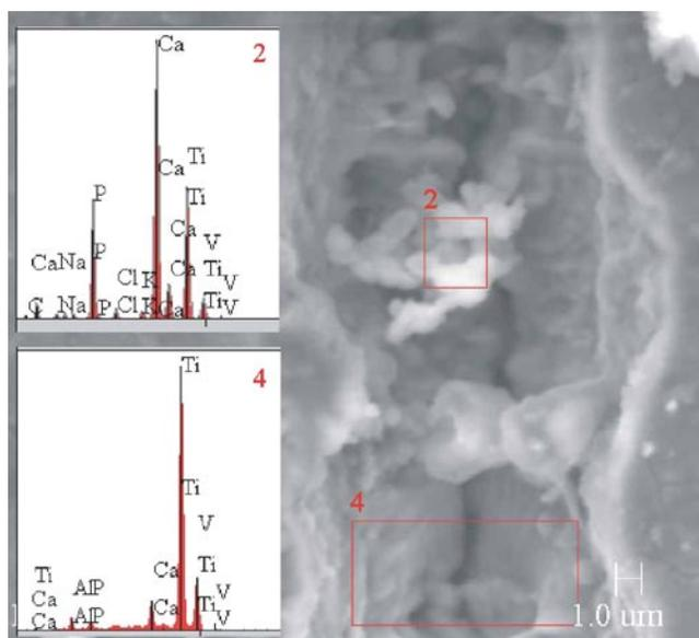
Fig. 5. SEM microphotograph and EDS results of EDS analysis for Ca-O-P deposits in the tensile stress zone of rebent specimen (bending angle 20°) after 30 days in SBF solution (5500x) [3]
