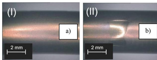
Fig. 2. Surface appearance after bending (angle 20°): a) zone (I) and b) zone (II) before immersion in Ringer's solution
